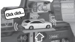
When dropping the elevator, please switch the Electric Screwdriver rotation to the opposite direction.
